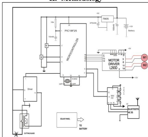
Figure1: Block Diagram of solar powered automatic lawn mower
